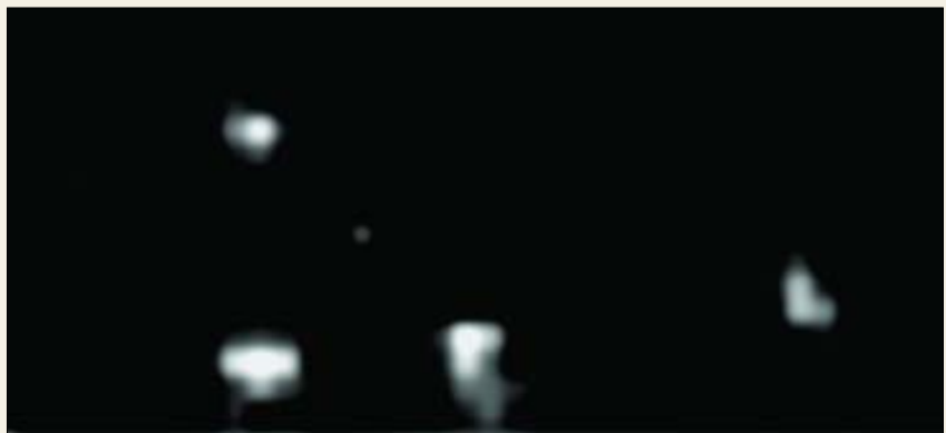
Figure 6. One frame of Footprints data (six-sensor mosaic), showing four people walking around. A mild filter was used to reduce visual artifacts caused by rectangles but the individual pixels are clearly visible. [Courtesy of R. H. Wolfe.]
