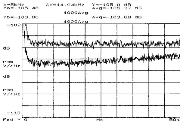
Fig. 11. Noise floor of the low-noise canceller of Fig. 10 compared with that of Fig. 4.  $Q_1$  and  $Q_2$  were part of a MAT-04 array, with five diode-connected (base and collector shorted) MAT-04 devices in each emitter. The value of  $i_{\text{signal}}$  was 0.189 mA and  $i_{\text{comp}}/i_{\text{signal}}$  was 5.0. The noise floor is 1.7 dB lower, in excellent agreement with the expected value of 1.75 dB calculated from Eq. (13).
