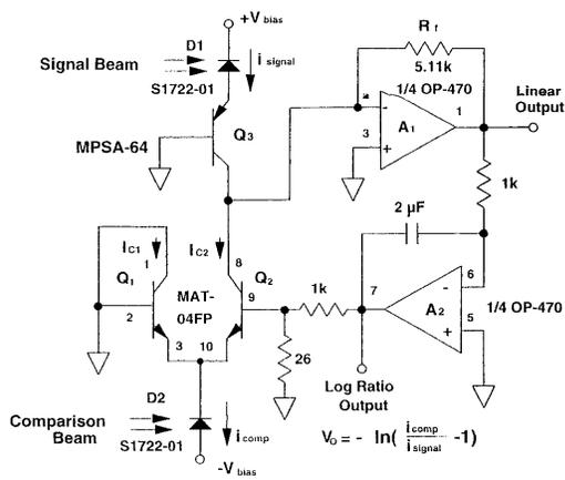
Fig. 3. Schematic diagram of the basic noise canceller. The BJT current divider  $Q_1/Q_2$  is controlled by servo amplifier  $A_2$  so that the dc output of transresistance amplifier  $A_1$  is zero. This ensures that  $i_{\text{signal}}$  and  $i_{C2}$  are equal. Because the fluctuations are proportional to the dc, the excess noise cancels identically at all frequencies of interest, independently of the feedback bandwidth.
