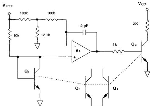
Fig. 17. On-chip temperature stabilization of  $Q_1/Q_2$ , which are diagonally opposite sections of a MAT-04. Of the other two sections,  $Q_5$  is a temperature sensor and  $Q_4$  a heater. The design temperature is 330 K with a reference voltage of approximately 5 V.
