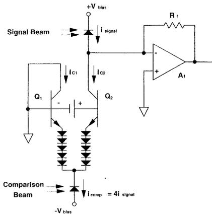
Fig. 10. One implementation of low-noise current splitting, to reduce the 3-dB noise penalty resulting from the uncorrelated shot noise of  $i_{C2}$  and  $i_{\text{signal}}$ . With  $i_{\text{comp}} = 5i_{\text{signal}}$ , the noise degradation resulting from  $i_{\text{comp}}$  is now a factor of 1.33 (1.25 dB) instead of 2 (3 dB) and can be reduced further by one increasing the relative size of the comparison beam.
