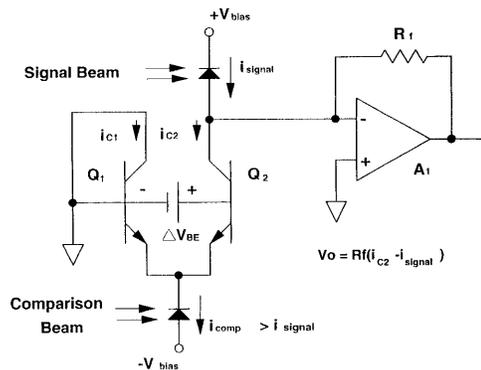
Fig. 2. Simplified schematic diagram showing the use of a BJT differential pair as a variable current splitter. The splitting ratio depends on  $\Delta V_{BE}$  but not on  $i_{comp}$ , so the fluctuations split just the same way as the dc.
