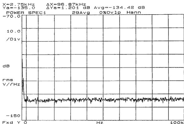
Fig. 21. Noise floor of the differential noise canceller of Fig. 19 ( $i_{\text{sig}1} = 1.83$  mA,  $i_{\text{sig}2} = 1.77$  mA,  $i_{\text{comp}} = 0.15$  mA). The total signal beam power was 14 mW. The available signal from  $A_1$  is 18.6 V, or +25.4 dBV. The measured 3–100-kHz noise voltage spectral density is -134.4 dBV rms/Hz or -134.6 dBV rms after correction for the 30-nV/ $\sqrt{\text{Hz}}$  instrument noise. The 1-Hz SNR is thus 160.0 dB.
