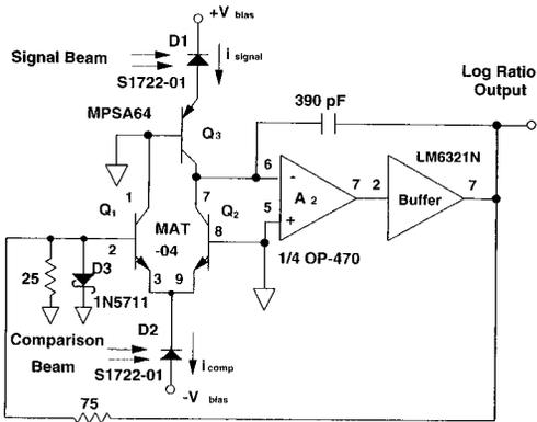
Fig. 14. Ratio-only version of the noise canceler. The photocurrent now goes directly to the summing junction of  $A_2$ . The time constant of  $A_2$  has been reduced. Feedback goes to the base of  $Q_1$  now, since the sign of the loop gain was changed by the elimination of inverting amplifier  $A_1$ . Schottky diode  $D_3$  protects  $Q_1$  from excessive base currents when  $A_1$  is saturated.
