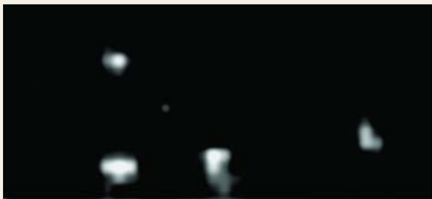
Figure 6. One frame of Footprints data (six-sensor mosaic), showing four people walking around. A mild filter was used to reduce visual artifacts caused by rectangles but the individual pixels are clearly visible. [Courtesy of R. H. Wolfe.]
