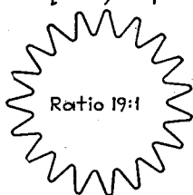
(c) Gear-wheel patterns obtained by inserting high frequency at point B to modulate sensitivity
