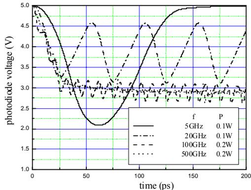
Fig. 6. The photodiode response obtained by SPICE on sinusoidal excitation for different frequencies of input signal.
