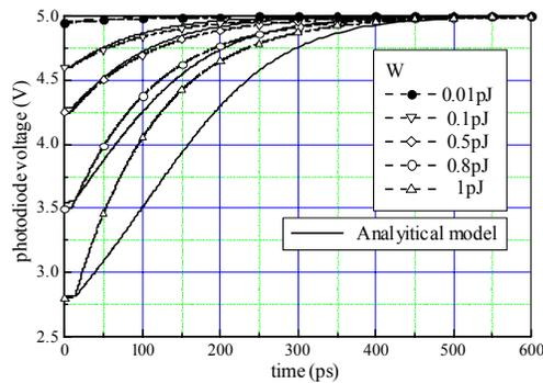
Fig. 2. The photodiode response on Dirac's excitation for the case of constant mobility of electrons. Comparison of SPICE results and analytically derived results [6]. Parasitic capacitance is  $C_s = 1pF$ .
