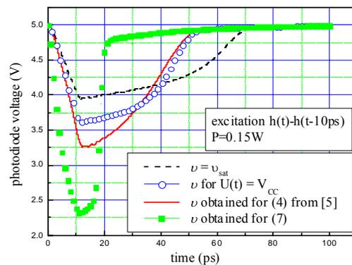
Fig. 5. The photodiode response on Heaviside's excitation. Dashed curve represents the results obtained from the velocity of electrons taken as constant equal to saturation velocity. Circular curve is obtained when we take form (4) from [5] but counting  $U(t) = V_{cc}$ . Full curve is obtained for (4) from [5] where we take into account change of  $U(t)$ . The last curve is obtained for constant mobility of electrons.
