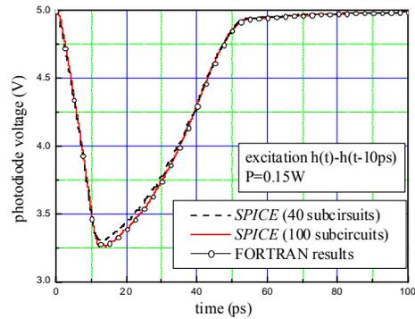
Fig. 4. The photodiode response on Heaviside's excitation. Comparison of SPICE results with 40, SPICE with 100 subcircuits and FORTRAN results.
