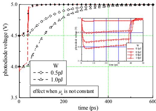
Fig. 3. The photodiode response on Dirac's excitation obtained with form (4) from [5]. Parasitic capacitance are  $C_s = 1pF$  and  $C_s = 0pF$ . Small picture presents the same results shown in another dimension.
