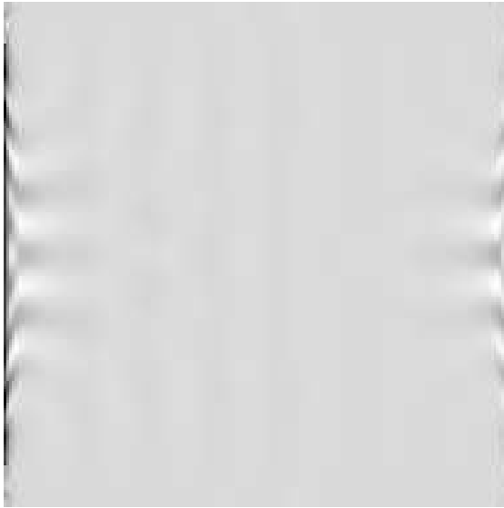
Figure 2.3 TEMPEST divergence due to source inside PML. This box is 3.2 wavelengths across.
